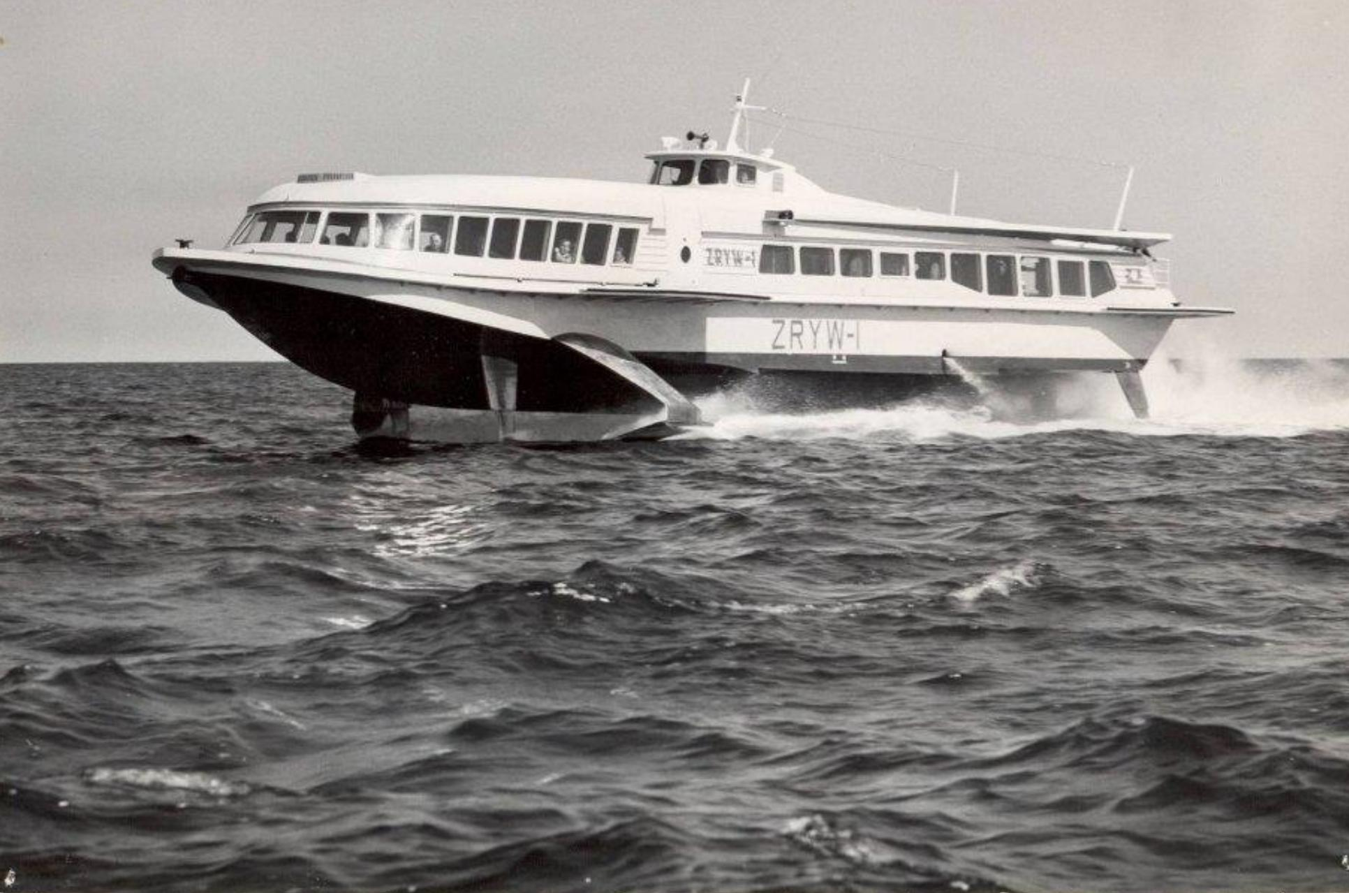
**„ZRYW” - Hydrofoil – sea going vehicle (L=27.6m; speed 35 knots=65 km/h)
