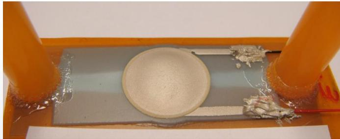
Flexible printed micropump on Kapton
